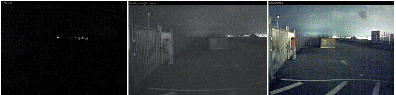
Lightfinder technology with AXIS Q1602/-E, AXIS Q1614/-E Network Cameras Left: Reference image, Middle: High-end surveillance camera, Right: AXIS Q1602/-E Network Cameras
